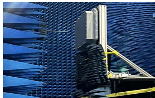
(b) 복사소자조립체 근접전계 시험 구성 (b) Configuration of near-field measurement for array radiator assembly
